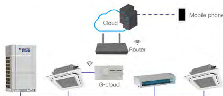
One G-cloud can control up to 80 sets of indoor units within one system
